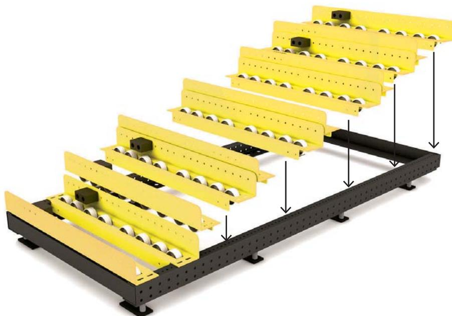
**STEP 14: Backstops are required for longer batteries.**
