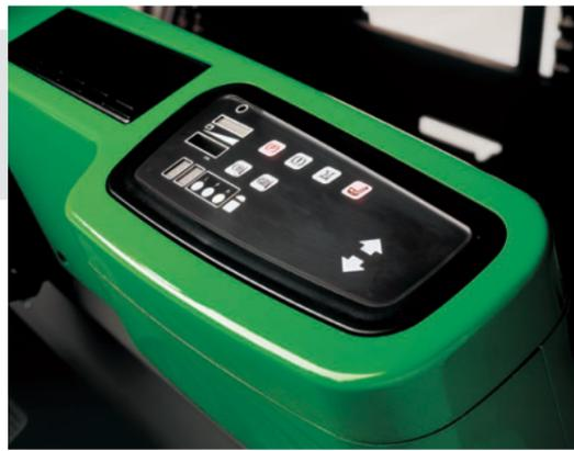
The automobile-style dashboard has main function indicator lights plus warning signals for operating faults and major component wear.
