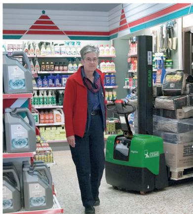
Climber wheels with single wheels are standard. These allow the truck to negotiate with ease obstacles such as pallets frames or trucks' ramps. The In-vehicle charging option, allows the truck to be charged during transportation if the lorry is configured with this option.
